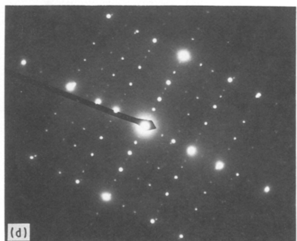
Figure 3 SAED patterns from the icosahedral quasicrystalline phase, I-phase. (a) Incident beam parallel to five-fold axis; (b) incident beam parallel to three-fold axis; (c) incident beam parallel to two-fold axis; (d) incident beam parallel to two-fold axis.
